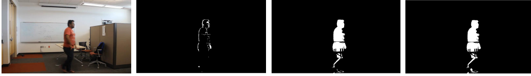
Figure 7.2: Figures from left to right represent the frame 1024, motion of the object in frame 1024 for offset 1, 20 and 124 respectively.
