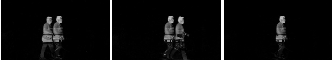
Figure 4.4: Figures from left to right represent the difference between frame 1030 and 1010, difference between frame 1030 and 1050 and motion of object in frame 1030 respectively.
